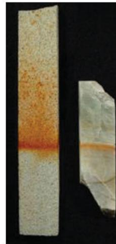
**Figure 4. Secondary mineralization on sandstone and albite coupons. Note higher staining at the scCO<sub>2</sub>/water interface.**
