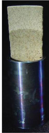
**Figure 2. High temperature rock coupon test specimens in individual titanium cups.**
